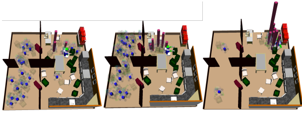
Figure 5: \hat{Q}(s, a) of PW-UCT, RAND-DOOT, and VOOT (left to right) after 50 visits to the place node for the first object. Blue and purple bars indicate values of infeasible and feasible placements, respectively. Solid robot indicates the current state of the robot, and the transparent robots indicate the placements sampled. Notice VOOT has far fewer samples in infeasible regions.
